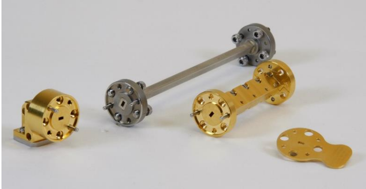
R 900 (WR 10) for 75 to 110 GHz: PCB adaptor, brazed w/g section, milled w/g section, \lambda/4 -shim (SPINNER GmbH, Munich, Germany)
