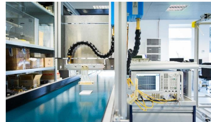
Flexible dielectric w/g with integrated transitions to R 900 (WR 10) metallic w/g (60 cm, 75 to 110 GHz, SPINNER GmbH, Munich, Germany, [10])
