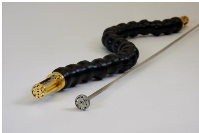
Flexible dielectric w/g with integrated transitions to R 900 (WR 10) metallic w/g (60 cm, 75 to 110 GHz, SPINNER GmbH, Munich, Germany, [10])
